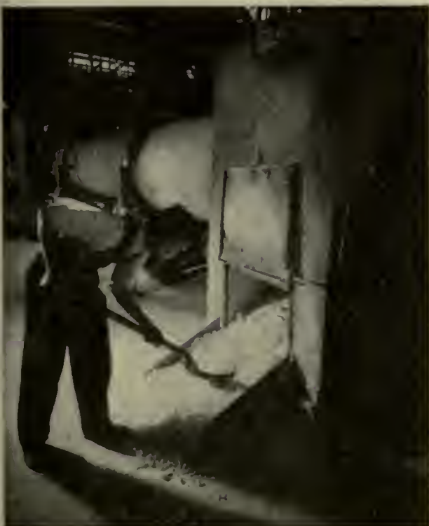
In this kiln aluminum sulphate is reduced to alumina
